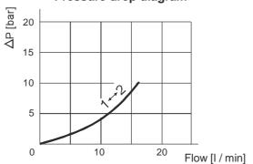
Note: Values measured on valve alone (no cavity) with an oil viscosity of 46 cSt at 50  $^{\circ}$ C. Pressure drop may change depending on fluid viscosity and temperature
