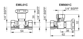
Weight: 0,14 Kg. Max working pressure: bar
