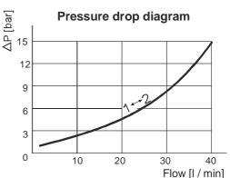
Recommended tightening torque: 45 Nm Recommended filtration settings: 25  $\div$  50  $\mu$  Oil temperature: -30  $\div$  + 80  $^{\circ}C$
