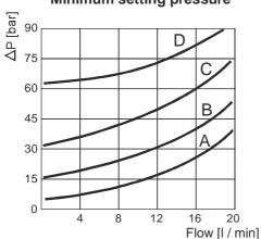
Note: Values measured on valve alone (no cavity) with an oil viscosity of 46 cSt at 50  $^{\circ}$ C. Pressure drop may change depending on fluid viscosity and temperature
