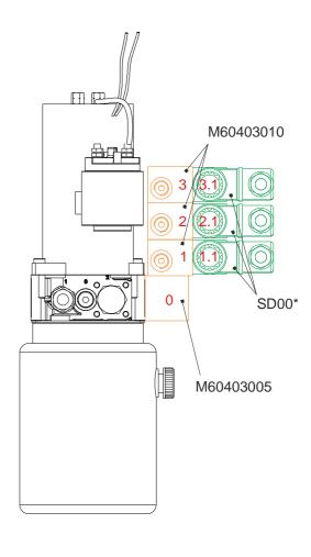
The micro powerpacks external manifolds and valves are arranged following a stack levels logic. Each stack is numbered as n, n.1, n.2, n.3,... where n is the basic manifold stack number, n.1 is the first valve mounted on top of manifold n, n.2 is the second one, mounted on top of n.1 one,...
