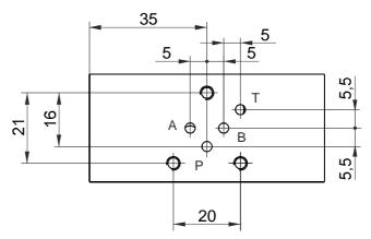
Weight: 0,21 kg Fixing system: 2 x M8 tie-rods steel class 8.8 or above
