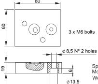
Spare part code: **N50403007** Mounting bolts 2 x M8x20 Weight: 0,22 Kg
