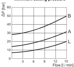
Note: Values measured on valve alone (no cavity) with an oil viscosity of 46 cSt at 50 °C. Pressure drop may change depending on fluid viscosity and temperature
