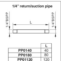
Recommended as suction pipe for PMC02 hand pumps and as return pipe with C3420001 return filter.
