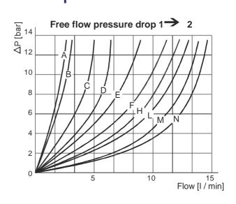
Note: Values measured on valve alone (no cavity) with an oil viscosity of 46 cSt at 40  $^{\circ}$ C. Pressure drop may change depending on fluid viscosity and temperature
