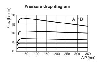
Note: Values measured on valve alone (no cavity) with an oil viscosity of 46 cSt at 50 °C. Pressure drop may change depending on fluid viscosity and temperature
