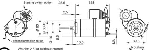
Permanent magnets Protection degree: IP54 Insulation class: F
