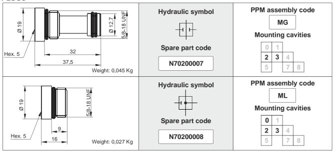
Note: cavities 2 and 3 are machined SAE08 (3/4-16UNF) in central manifold MB and 5/8-18UNF in central manifold MR. Cavity 2 is machined SAE08-4way in central manifold M4.
