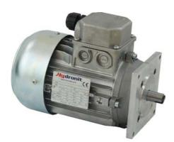
B14 IEC standard AC motors: the standard solution easily available on every market from 0,12 to 0,55 kW, single or three phase. These motors are normally procured by the customer itself. Hydronit provides adaptor flanges and double piece coupling for frame size: 63 and 71.
